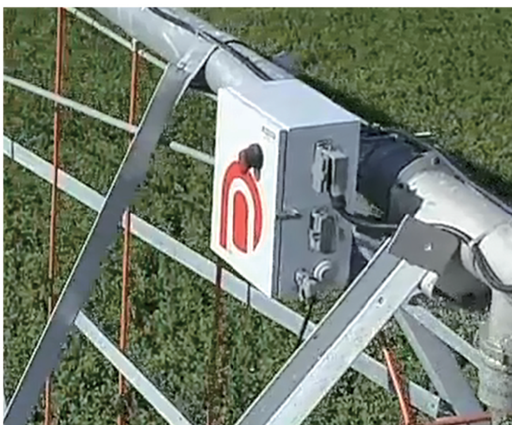
Patented VFD tower boxes -drive pivot constant move instead of start-stop move
