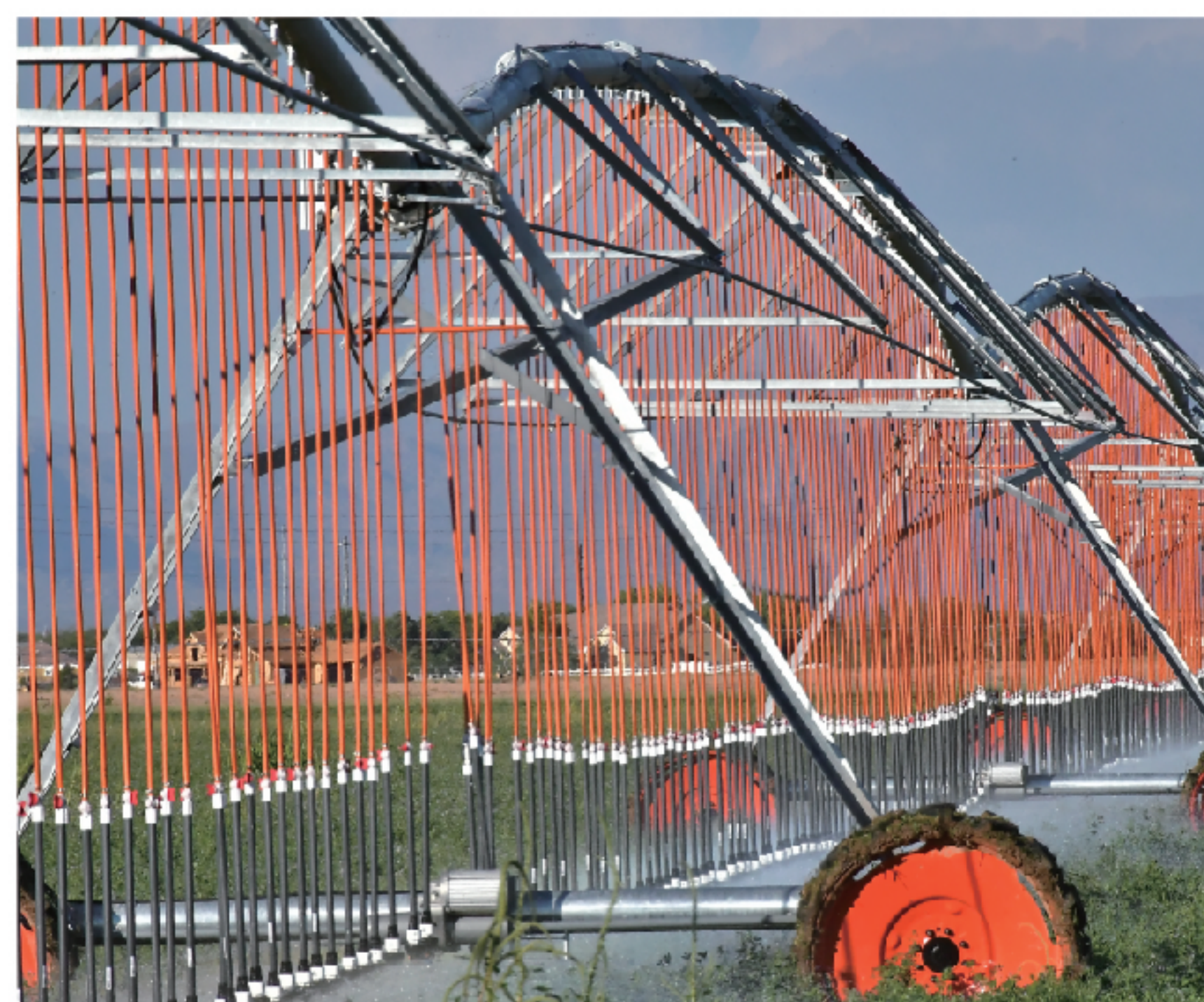
30" spacing outlets design, much better uniformity liquid application.
