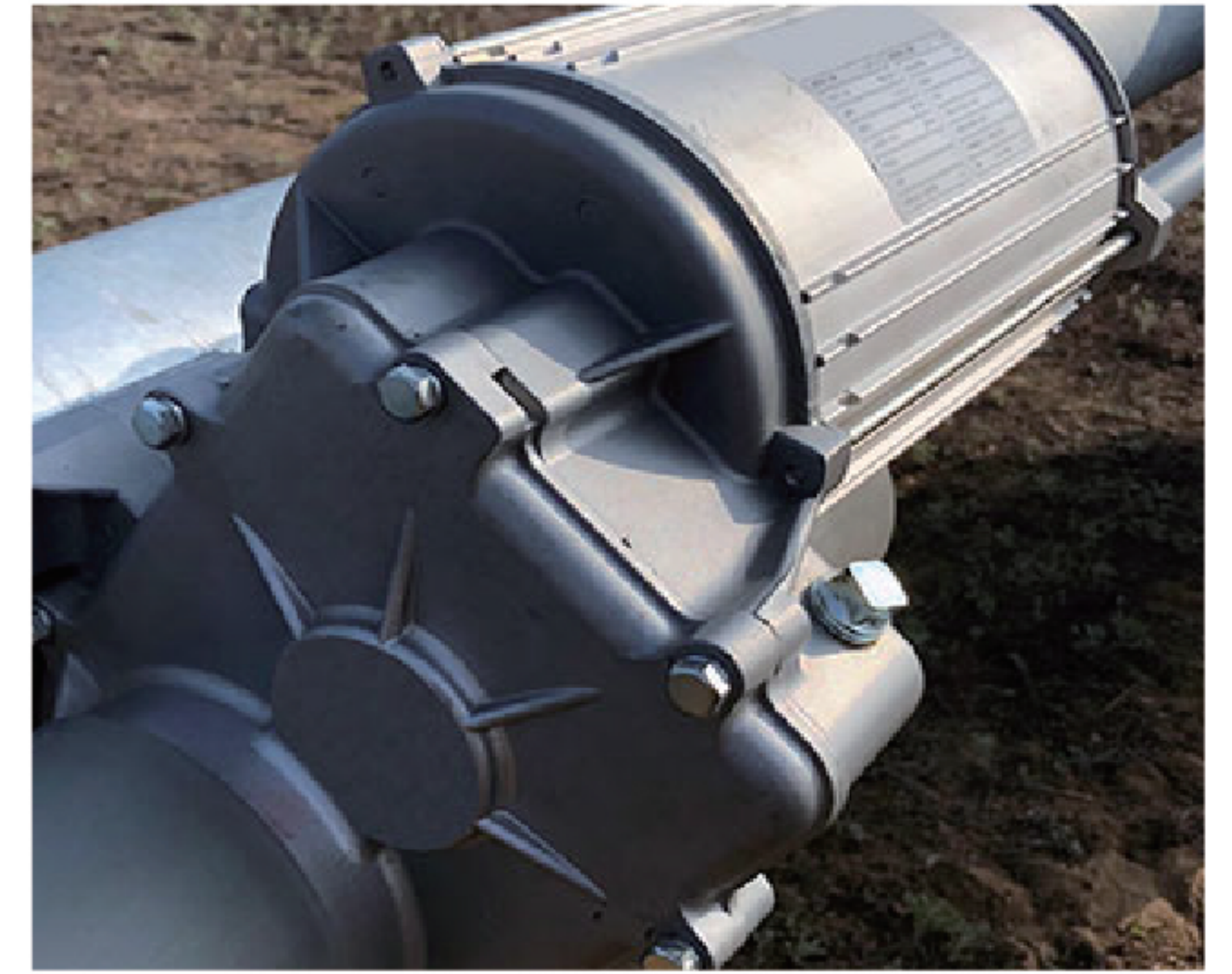
Center drive 3.5 hp/10:1- drive pivot wheels maximum speed 7.2 RPM .
